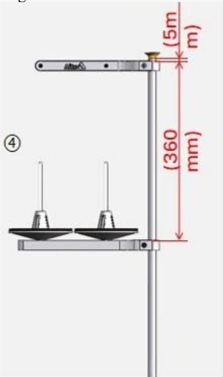
Fig. 2.7 Recommended Height of Line Frame Pole
